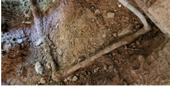
Excavation of the water supply pipe revealed it to be heavily corroded across a 2-metre section
