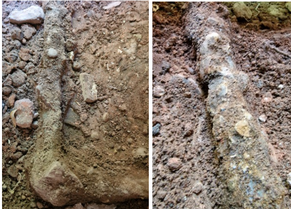
Stones were imbedded in the pipe, leaving craters when removed in addition to existing leak points
