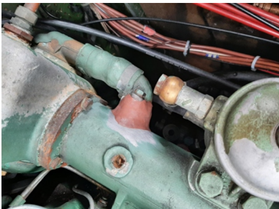
The hole was sealed by total encompassment with Superfast Titanium
