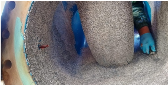
WearShield created a 30mm thick alumina-reinforced protective shell over the pump housing
