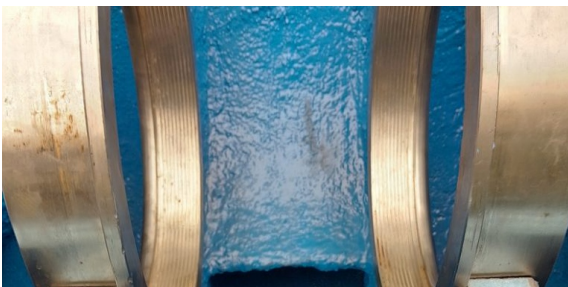
Top coating WearShield with Ceramic Brushable left an ultra-smooth, low-friction finish to the repair
