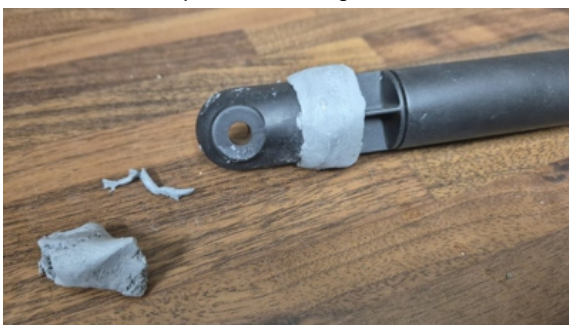
A further ring of Superfast Aluminium was applied around the break area following reassembly for added reinforcement
