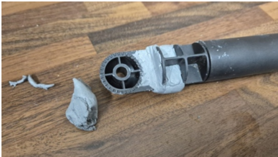
Superfast Aluminium was shape to mechanically bond the broken pieces back together
