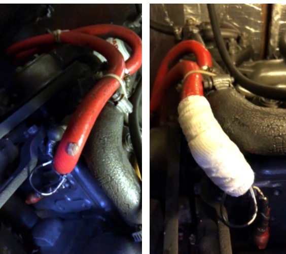
Superfast Steel was applied to the pinhole, followed by a SylWrap HD Bandage to seal the leak
