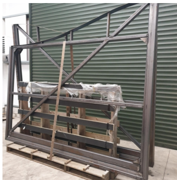
The steel frame to which the slats would be fitted
