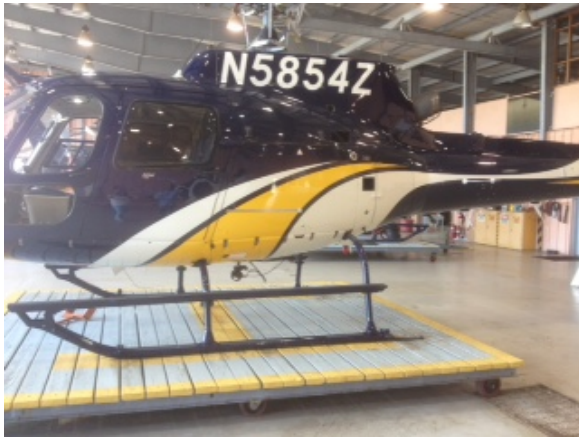
A helicopter belonging to the Puerto Rico Power Authority. Some maintenance jobs involved workers standing on the legs of the helicopter, which had anti slip tape applied as a means of protection
