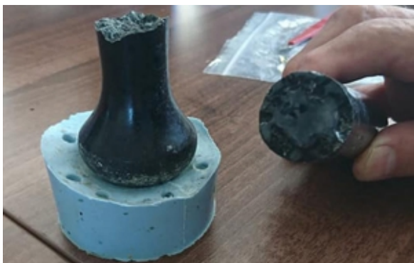
The bottom section was held in place with rubber. The top section was coated with Rapid 5 Minute
