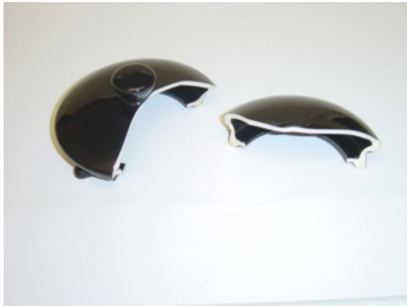
The teapot lid cracked into two separate pieces. The break joint was a complex shape, meaning the repair needed an epoxy adhesive with a long enough work time to be applied rather than the instant bond of a traditional superglue
