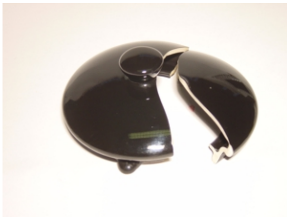
The two parts were pushed together once one side of the break had been coated with epoxy. A five minute cure time allowed the pieces to be adjusted for a seamless fit
