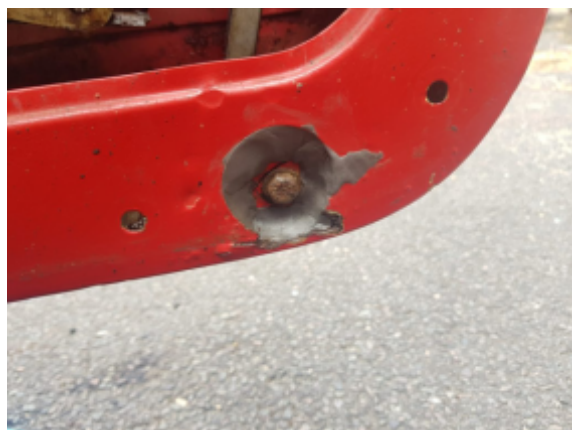
Superfast Steel was pushed into the hole and shaped around the screw, filling the damage. Once cured, it was filed and painted red to match the car frame
