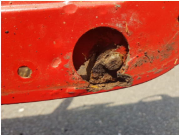
Corrosion had eaten away at the metal frame of the car, causing rust holes to develop around a screw
