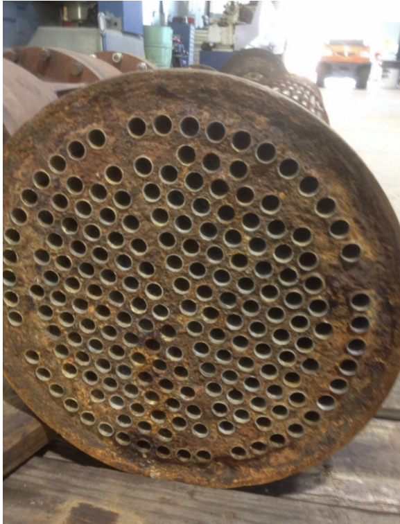
The cast iron face of the condenser unit suffering from heavy corrosion after 20 years of service
