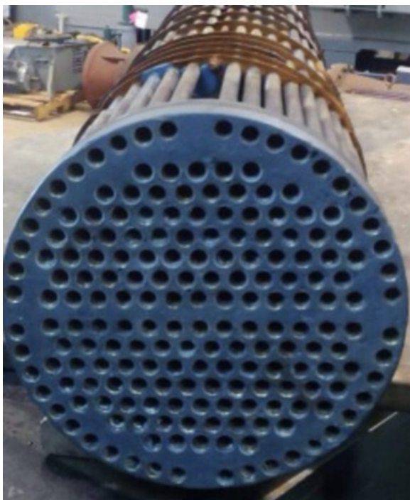
Ceramic Supergrade rebuilt the face, creating an ultra-smooth surface with high corrosion resistance
