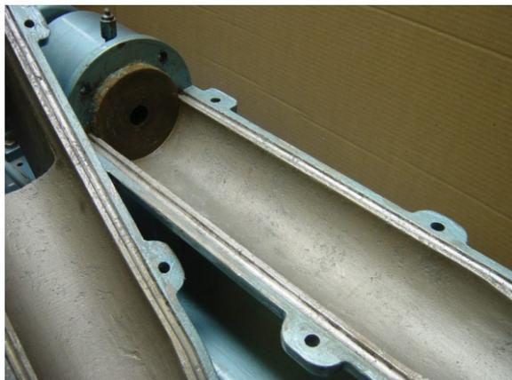
*Aluminium barrels in the putty extruders suffering from wear which was impacting on efficiency*
