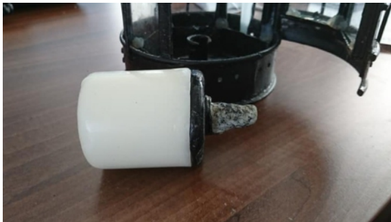
Superfast Steel was formed into a new platform and spike capable of holding larger candles
