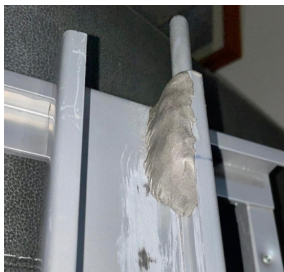
Pin permanently reattached to the unit, avoiding the £290 cost of buying a replacement magic corner
