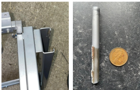
Part of the unit from where the 100mm pin snapped off and the pin itself once detached from the unit
