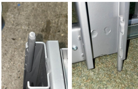
How the pin would have looked when welded to the magic corner unit prior to snapping off
