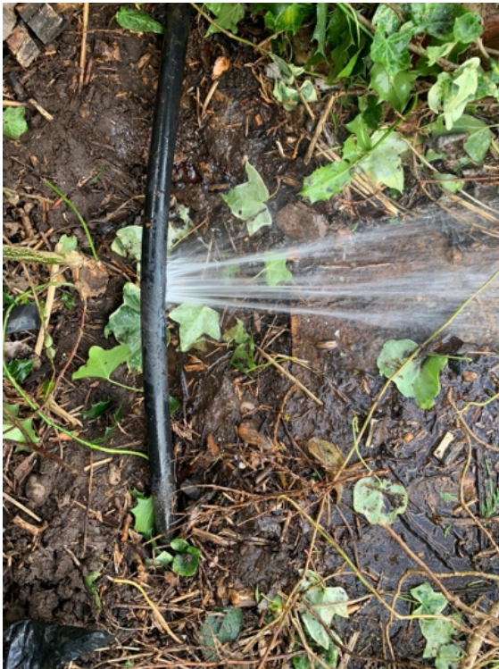
Water escaping from 80mm split in the hose
