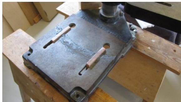
Industrial Metal was applied with a hand tool to rebuild the damaged area of the stand
