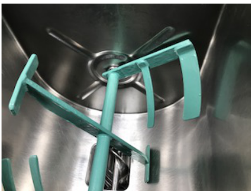
The corroded blades inside the mixers after the application of Ceramic Brushable Green
