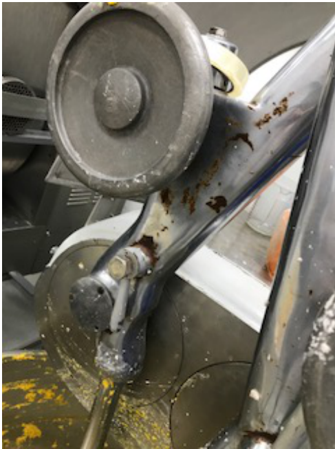
An example of the sort of corrosion which the flour mixer was suffering from prior to repair
