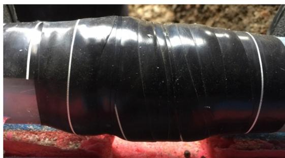
Wrap & Seal sealed the hole with a temperature resistant repair
