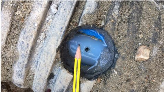
The pinhole caused when the pipe was cut into
