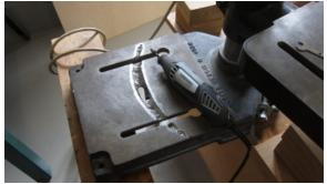
Deep gouge in the drill base stand caused by misuse
