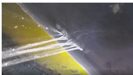
The 50mm crack in the pipe facing towards ground
